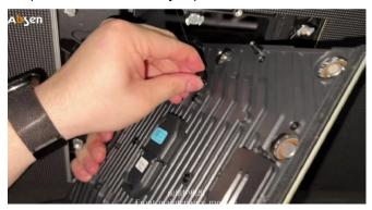
Step3: Remove the failure module.
