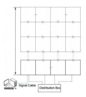
This product cannot store or display video content solely on itself. To perform normal work, the screen requires video source from the output device such as PC, laptop, media a payer, etc. and one or more sending box to receive and feed the source to it.
