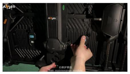
Step2: Replace with a good module and lock the safety rope.
