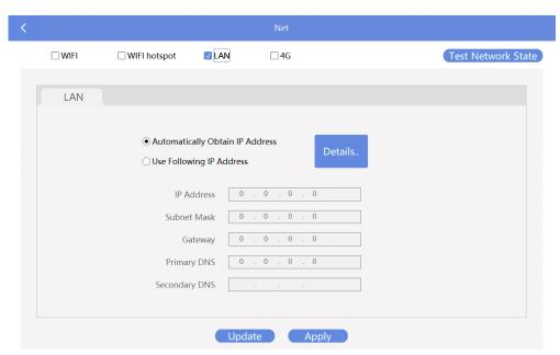
Take LAN port as an example. After it is connected to the network cable, the player will automatically obtain the IP address.
