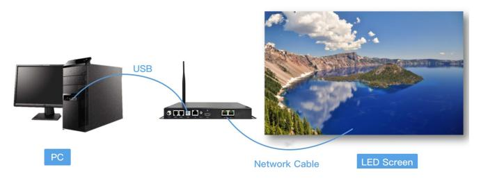
2. Configure LED display screen parameters and ensure that the display screen can display the complete picture
