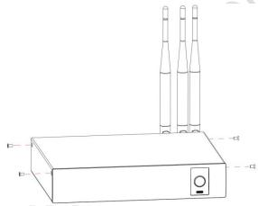
3. Align the rack ear holes with the device screw holes and secure them with screws.
