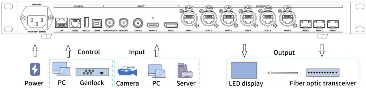
**Ethernet Port Output:** When using an Ethernet port board, the port is directly connected the LED screen via a network cable.
