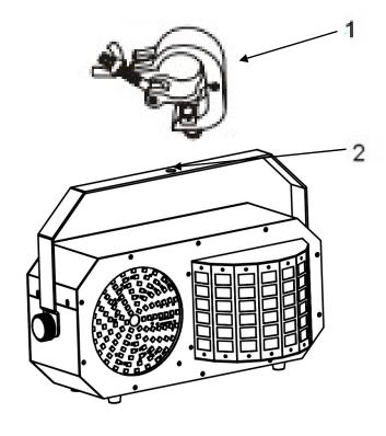
When install this equipment please make sure there's no flammable surfaces (decorated things, etc) within at least 2.5M and maintain minimum distance of 0.5M from the equipment to the walls.
