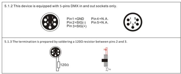
5.1.4 Connection: use DMX cable with 5 pin XLR-plugs to connect the controller with the fixture or one fixture with another.
