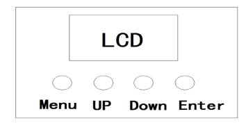
Menu – Move up a level. Up – Move selection up one item. Down – Move selection down one item. Enter – Select / Move down a level.
