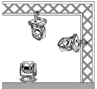
The device could be either put on a solid and even Surface, or mounted upside down or sideways like left picture.
