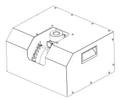
Place the silo into the spout and secure it with torx screws. (as shown below) The machine can adjust a total of 5 nozzle angles. Each Angle is 15 degrees apart. Before adjusting the Angle, please install the safety shaft to the position that needs to be adjusted, and then pull up the locating pin to adjust the nozzle Angle.
