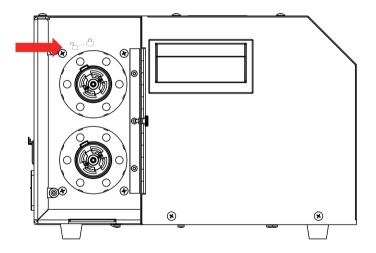
**CAUTION** If the tank can't be installed successfully, please check buckle is in the right place.
