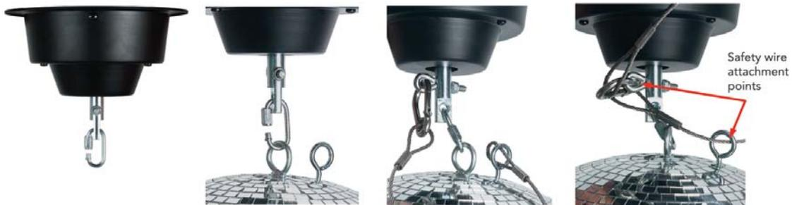
Attach mirror ball to motor axle using carabineer (not included) (make sure to close carabineer!). Attach safety wire to the mirror ball eyelet and the motor safety eyelet.
