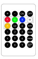
Press **Auto/Sound/Strobe** to switch on or off Auto mode, Sound Active mode and Strobe mode, respectively.
