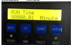
Note: Once the machine is started, the cumulative running time will be displayed automatically, including the actual spraying time but excluding the standby and warm-up time. The cumulative time is maximum 60000.00 minutes and accurate to a second. If the cumulative time exceeds 60,000 minutes, the system will automatically clear it and re-calculate the time, as shown below:
