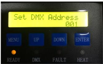
Press UP or DOWN to select a value between 1 and 512. Press ENTER to go back to the main menu or MENU to enter the temperature setting.
