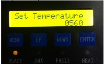
Press UP or DOWN to set the temperature between 560°C and 620°C. Then press ENTER or MENU to go back to the working status interface.
