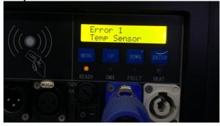
If the temperature sensor is in the normal status, warm-up will be started. The HEAT indicator will flash in the warm-up process. After warm-up, the HEAT indicator will be OFF.
